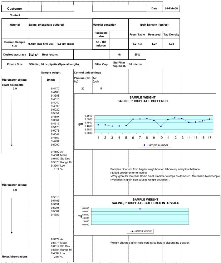
1. Free flowing powder with average angle of repose. Somewhat granular non uniform particulate material. Many clumps up to 1.5 mm dia. as delivered. Hydroscopic, moisture weight gain the longer the powder was exposed to the air.
